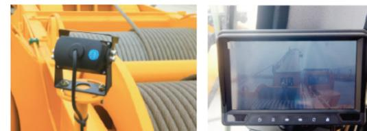
◎ The operator's cab is equipped with the winch monitor for easy observation and operation.
