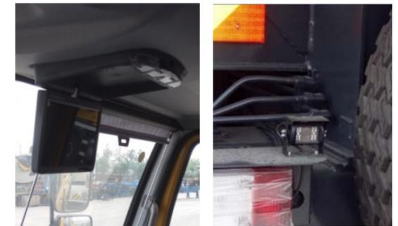
◎ The reverse image system is set in the cab to make parking easier and avoid scratches.
